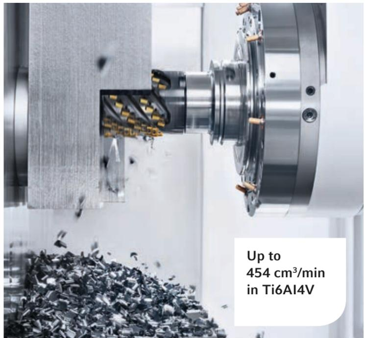
Up to 454 cm<sup>3</sup>/min in Ti6Al4V
