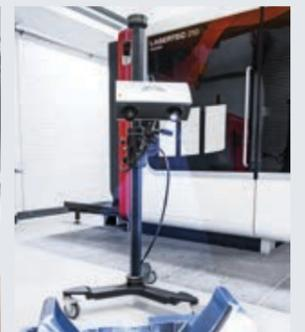
Measuring the mould geometry with a 3D scanner.
