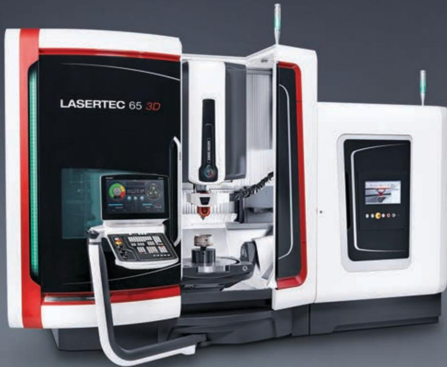
Flexible HSK interface LASER + Mill + ULTRASONIC\*
