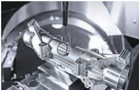
5-axis machining on a DMU 60 eVo.
