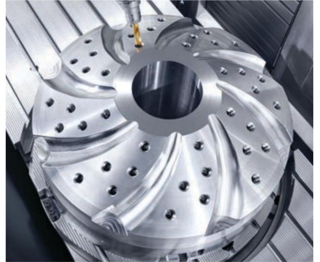
Integrated rotary table for 5-axis and mill-turn machining.
