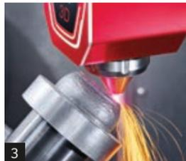
3 Laser deposition welding and milling combined on the LASERTEC 65 3D (flexible change possible).
