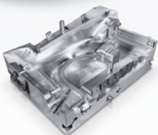
Press tool for car wings Machine: DMU 340 P Material: 1.2343 Dimensions: 1,000 x 1,800 x 400 mm
