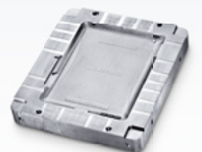
Injection mould for Tablet PC cover Machine: LASERTEC 75 Shape Material: Aluminum Dimensions: 290 x 220 x 65 mm
