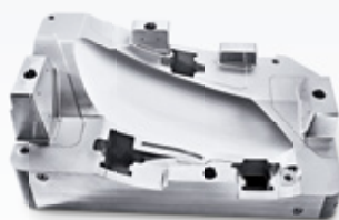
Injection mould for headlamps Machine: HSC 70 linear Material: 1.2312 Dimensions: 680 x 400 x 350 mm, Ra < 0.15 μm
