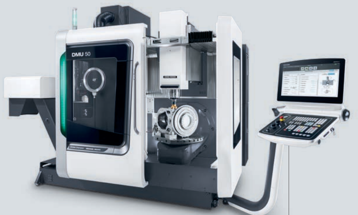
NC rotary table swivel range: -5° to +110°.
