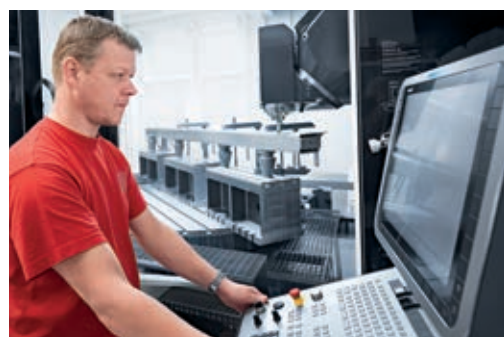
5-axis simultaneous machining of large components on the DMU 340 P.
