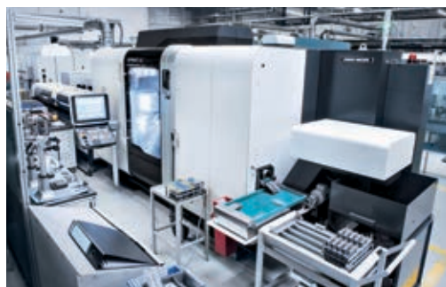
Production on the SPRINT 65 with unrivalled precision, e.g. flatness of 0.004 mm.
