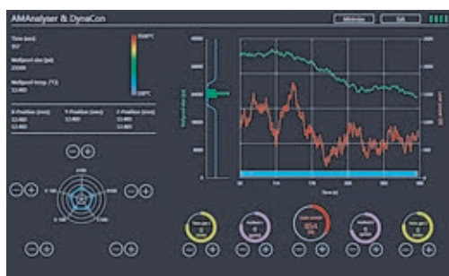
Adaptive process control Automatic adjustment of laser output.
