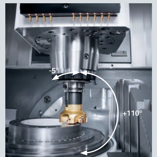
NC rotary table swivel range: -5° to +110°.
