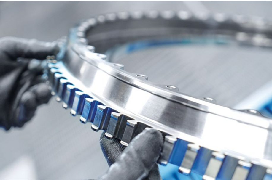
Quality control: Visual inspection of a turbine disk made from Inconel 718.
