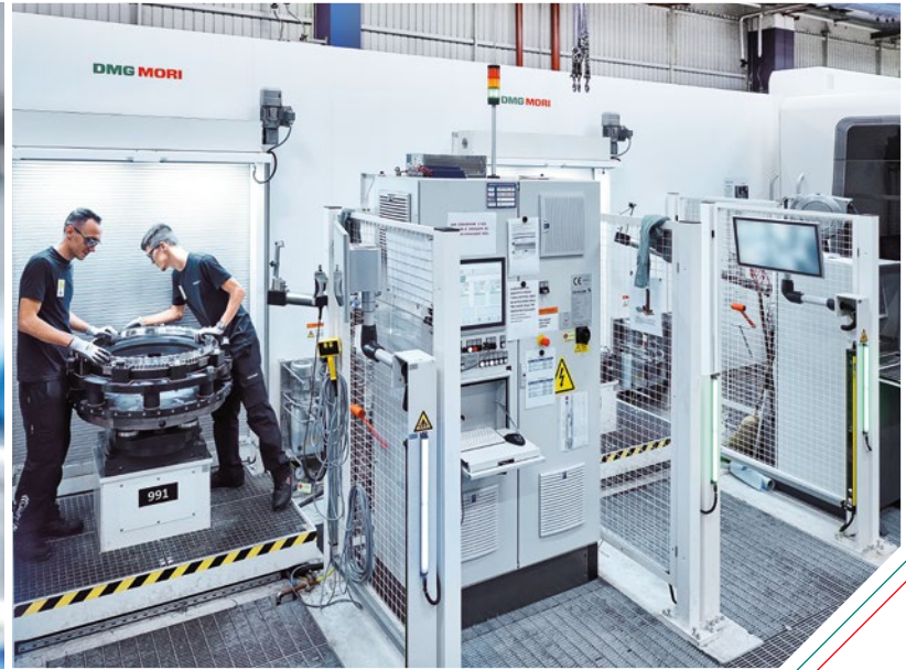
Setup station for the production line with the four DMU 80 FD duoBLOCKs.
