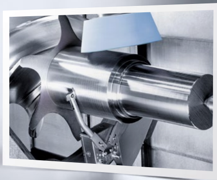
In-process gauging during grinding: Measuring repeatability 5 µm.
