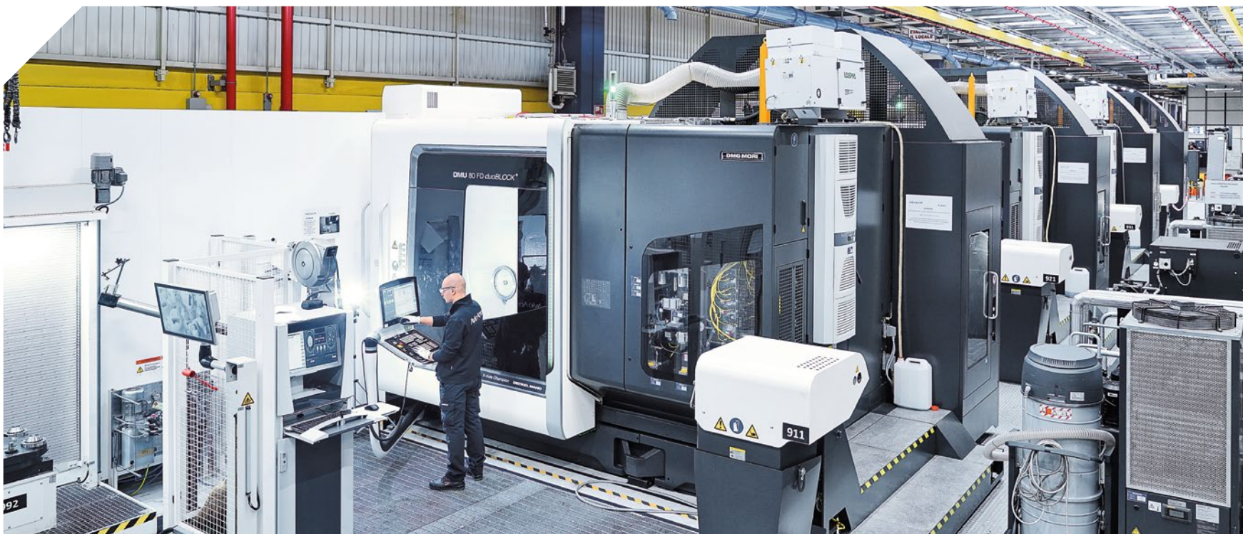
Customer-specific automation: Four automated DMU 80 FD duoBLOCKs linked to a pallet storage system.
