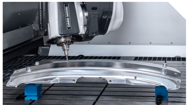
Die & Mold: 5-axis simultaneous machining of an aluminum mold insert.
