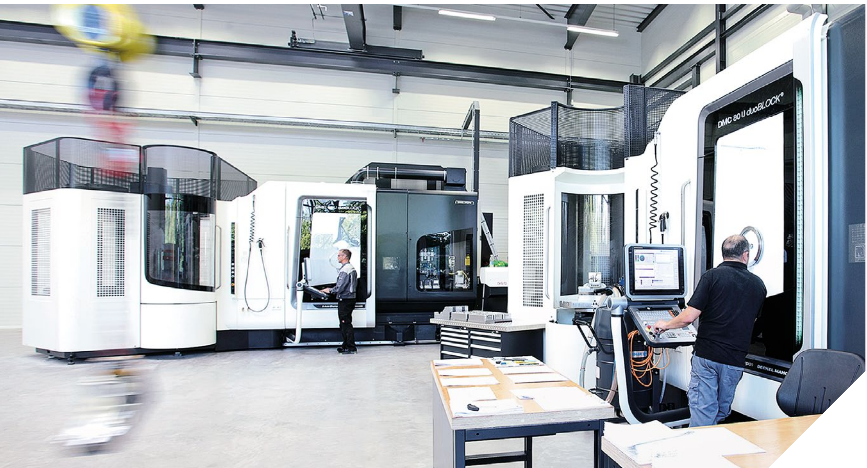
Equipped with RS 12 rotary storage units for up to twelve pallets, the two DMC 80 U duoBLOCK machines can work efficiently round the clock.
