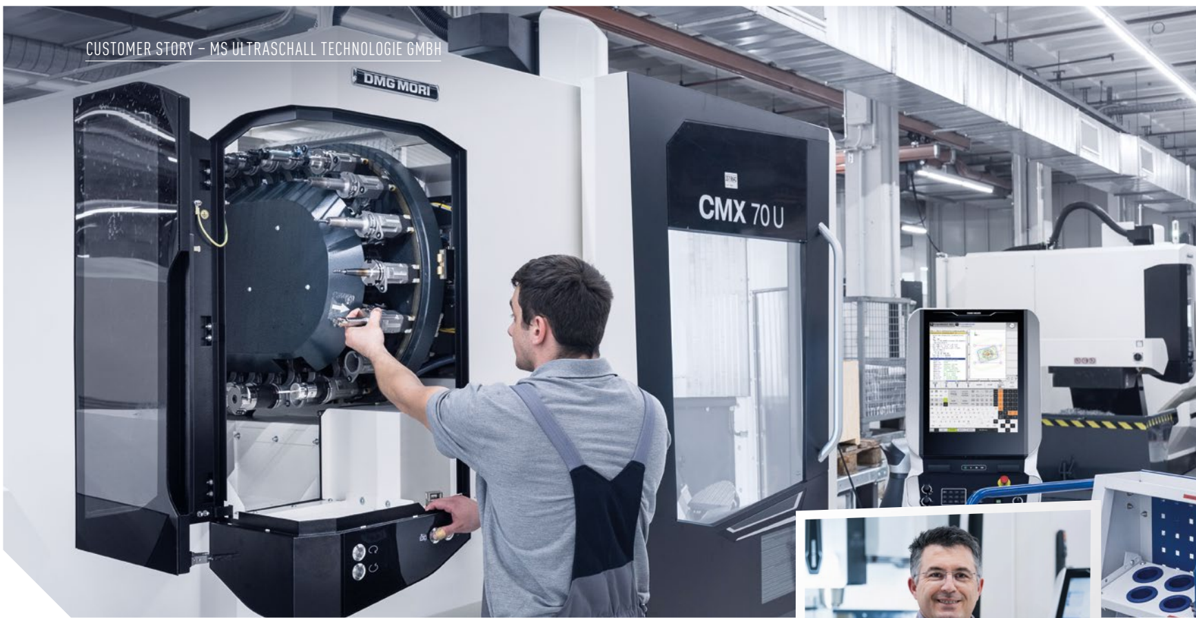
Setup during machining, thanks to a separately accessible tool magazine on a CMX 70 U.
