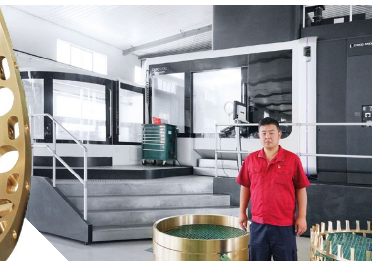
RUIGU production manager Mr. Chen in front of the DMC 210 U on which oversize bearing cages are manufactured.
