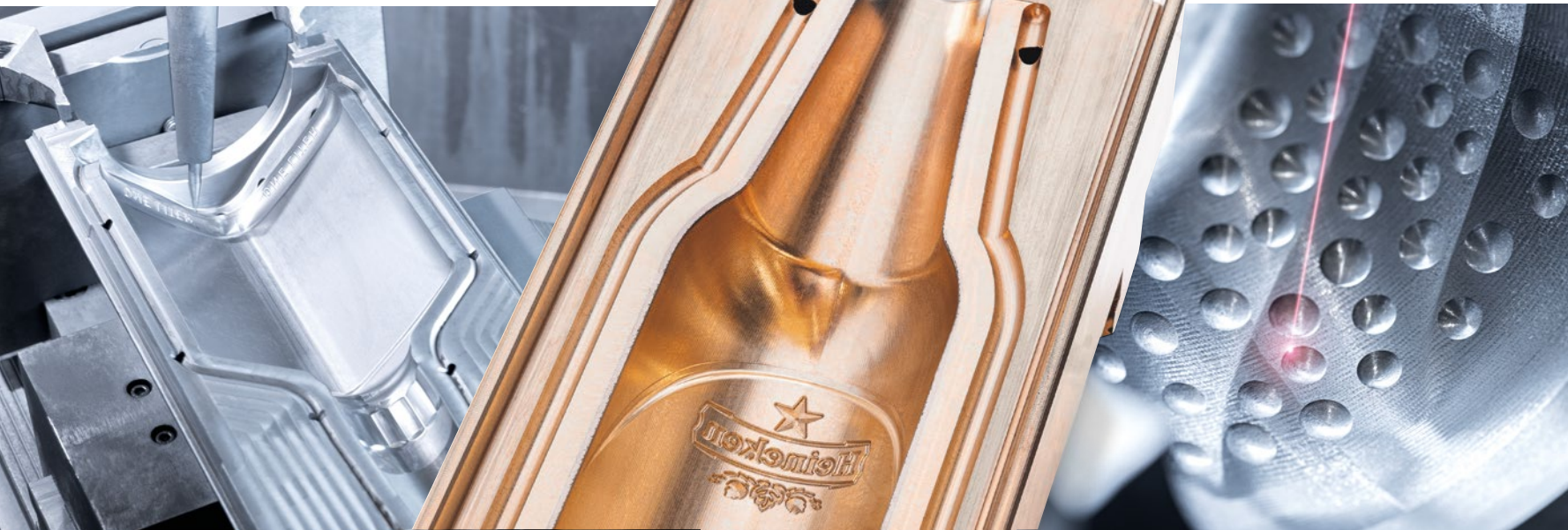
Using 180 DMG MORI machines – among them ten HSC 55 linear for high-speed cutting and five LASERTEC 45 Shape for surface structuring – OMCO manufactures highly precise glass molds.
