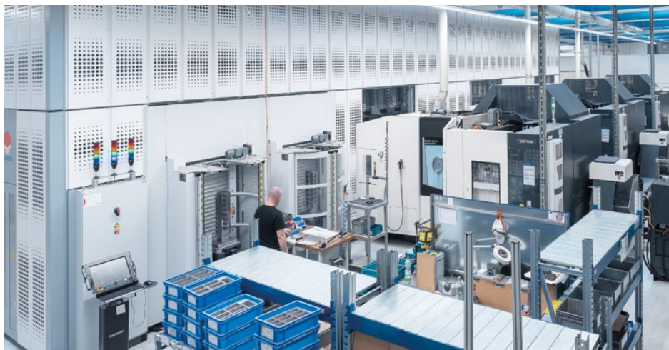
The largest of the automation systems installed to date includes three DMC 60 H machines each with a 5-wheel magazine for 303 tools.
