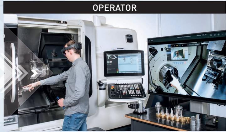
The trainer can optionally connect to your machine via the DMG MORI NETservice. This gives the trainer all the necessary machine information on a second screen.
