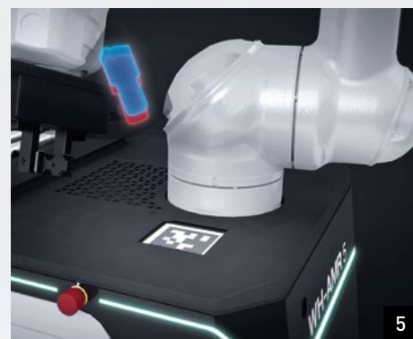
CPC function for position correction
