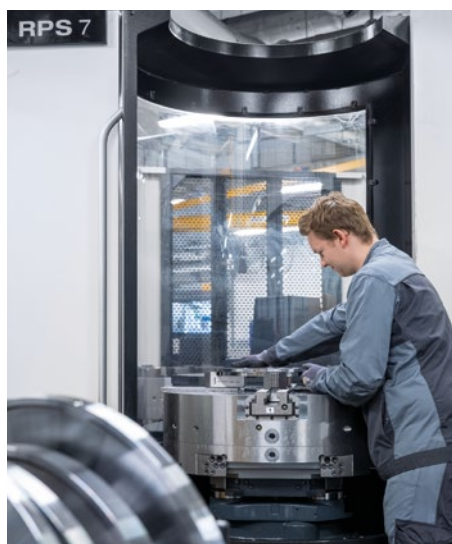
Electrically-actuated, intelligent chuck for highly sensitive component clamping.
