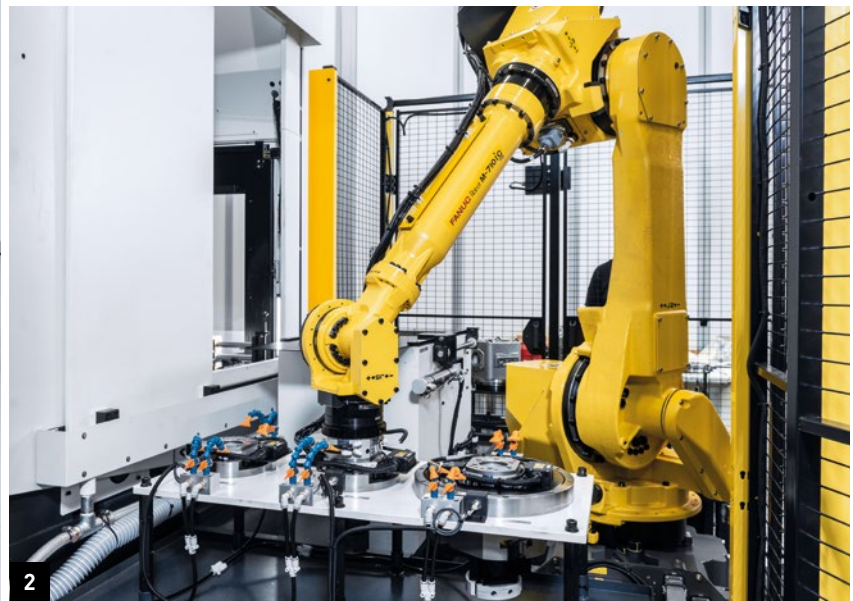
1. DMG MORI integrated a blow-off station in the automation, which cleans each component before and after machining 2. Thanks to the use of several grippers, Richter Feingerätebau can also machine different workpieces automatically
