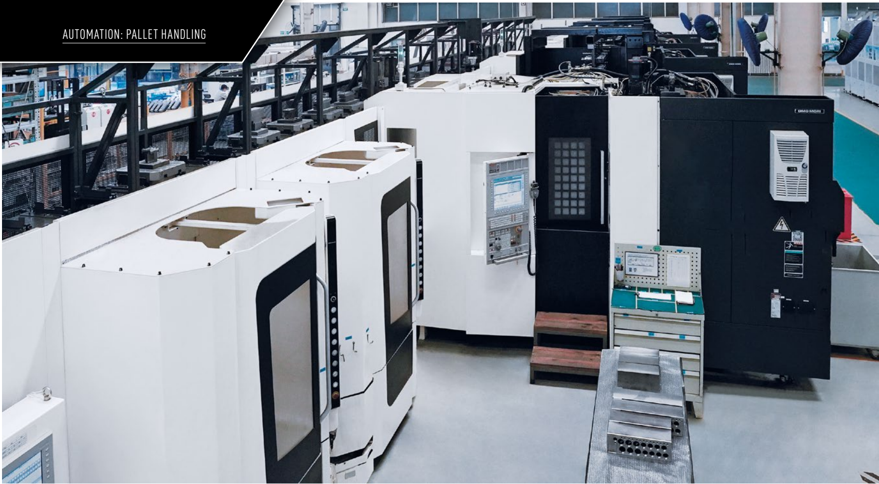
One of the LPP Systems: LPP with 48 pallet stations, 2 setup stations and 4 NH 5000 DCG.
