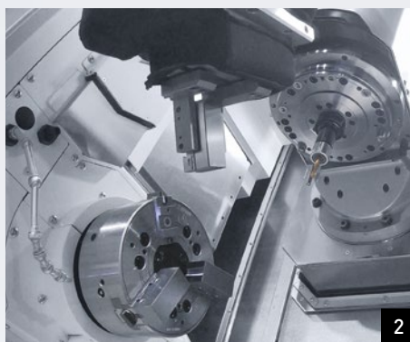
Can exchange chuck jaws inside the machine
