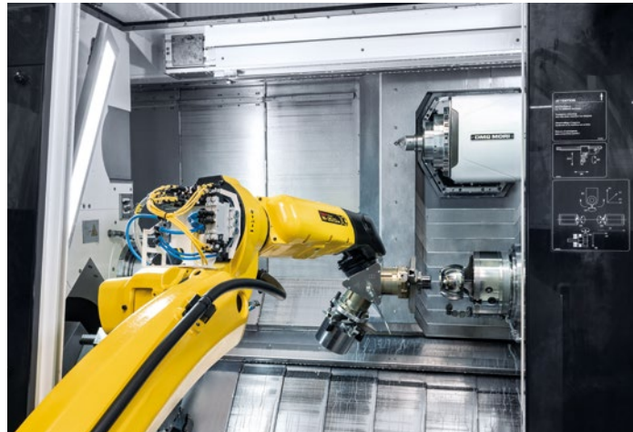
Simultaneous processing of two workpieces: As soon as machining at the main spindle is finished and the component has been transferred to the counter spindle using Robo2Go, a new unmachined billet is clamped.
