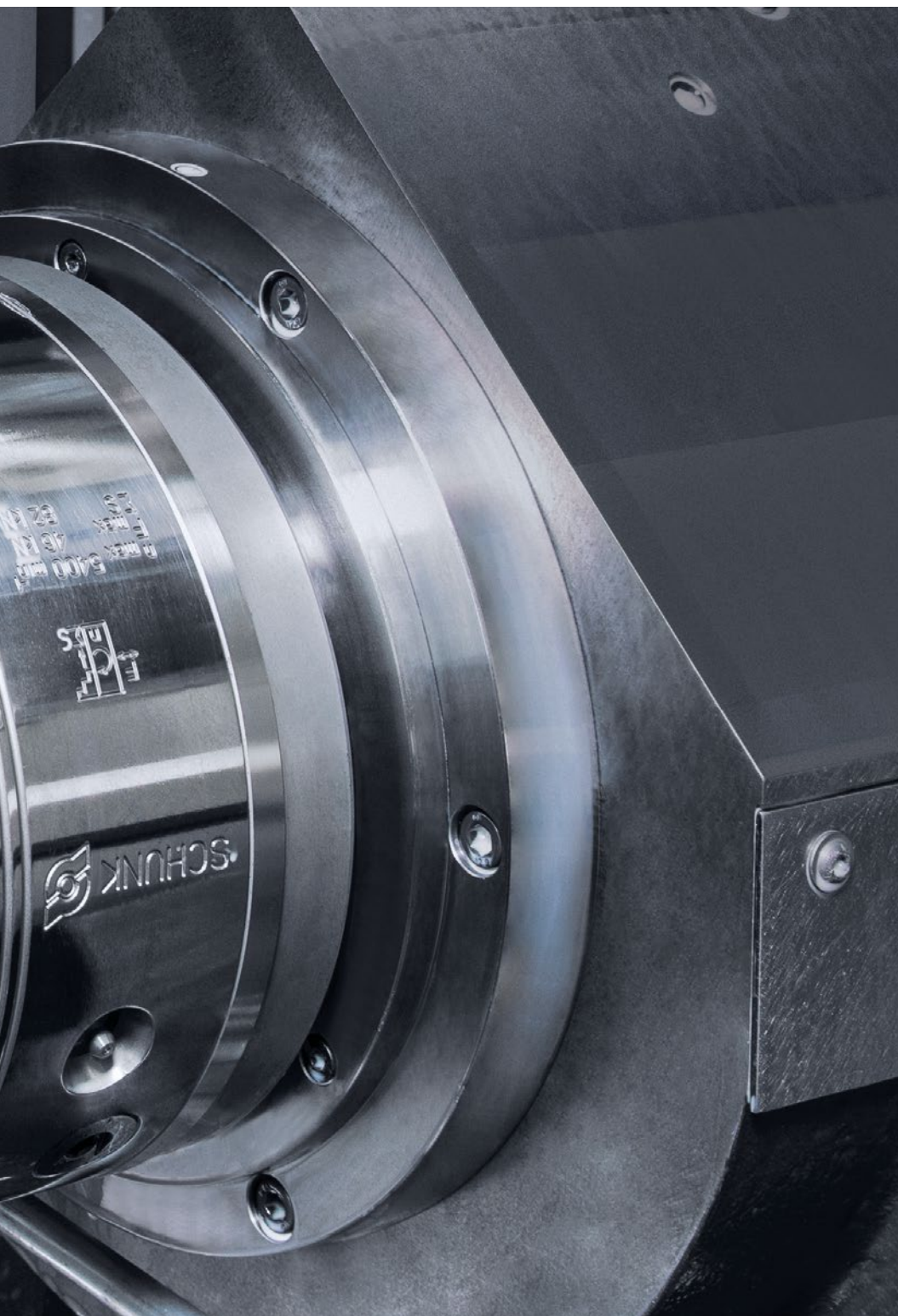
CTX beta 1250 TC 4A: With 6-sided turning and milling and simultaneous machining at two spindles, HÜBNER has been able to reduce throughput time by one quarter in comparison to the original process.
