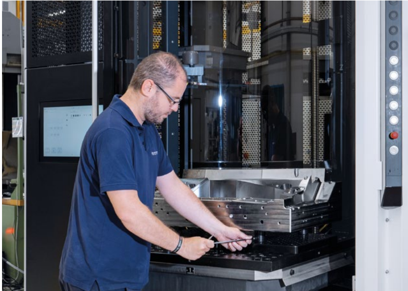
PH Cell 2000: We can prepare so many pallets here in parallel with production that machine downtime is minimal – even into the night.
