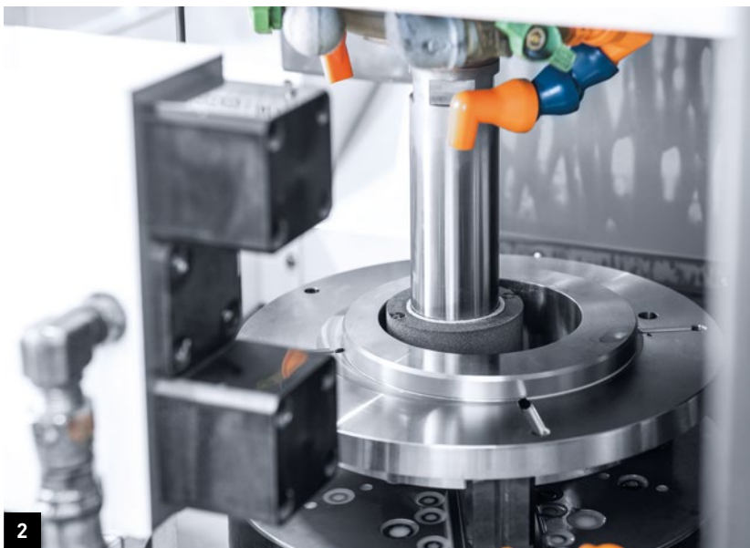
Thomas Strauß (right), authorized signatory of Richter Feingerätebau, and Horst Hoferichter, authorized signatory/technical management 2. Equipped with internal and external grinding spindles, the IGV-3NT enables the grinding of internal, external and flat surfaces in a single setup 3. In 2022, DMG MORI installed an IGV-3NT including an individually designed automation solution at Richter Feingerätebau 4. Every component is checked with a touch-probe after machining
