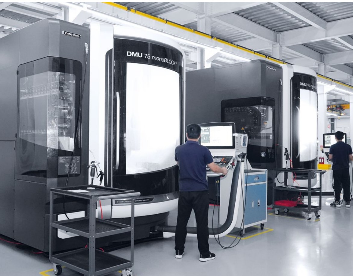
GRANDE-TEK has two DMU 75 monoBLOCK machines and one DMU 125 FD duoBLOCK for milling and mill-turning.
