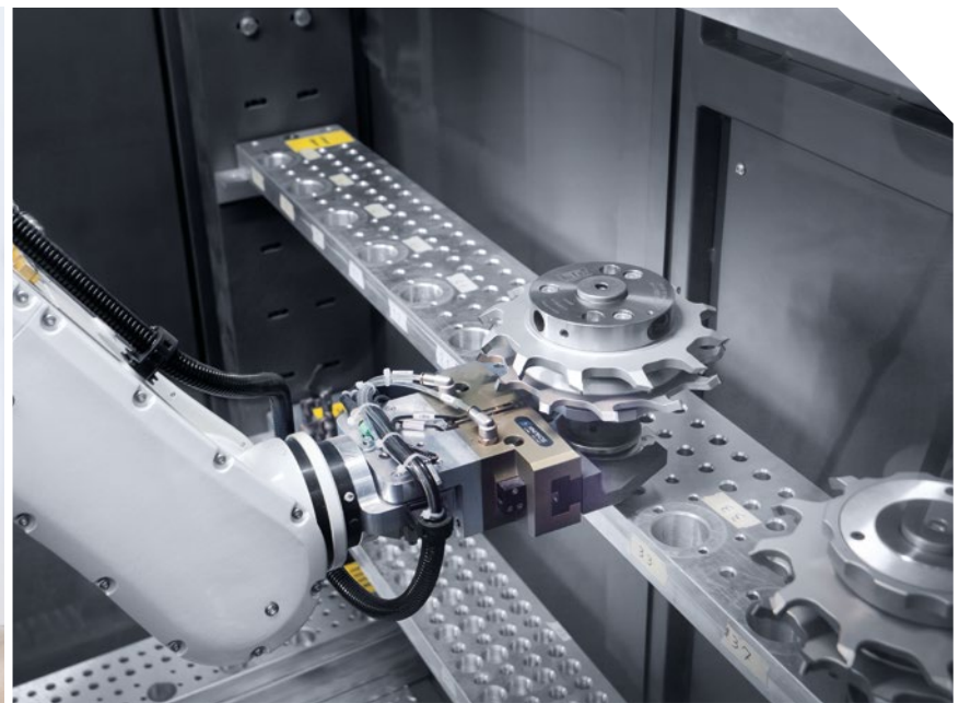
Maximum utilization in unattended multi-shift operation by means of automated component handling.
