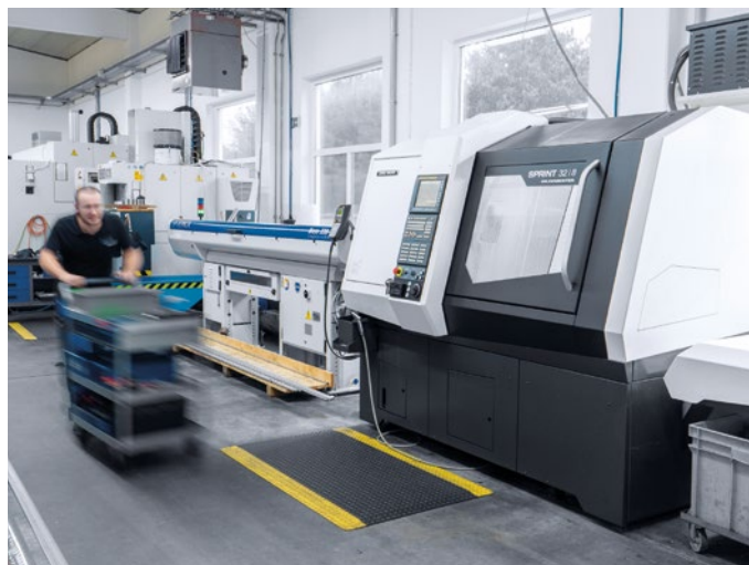
SPRINT 3218: Up to 28 tool locations on 2 independent linear tool carriers enable highly productive production of workpieces with a diameter of up to 32 mm.
