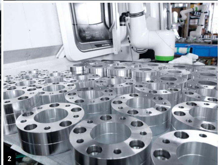
1. Main workpieces. The jaws for clamping the workpiece were also designed in-house. 2. Workpieces are stacked for long hours of continuous operation.
