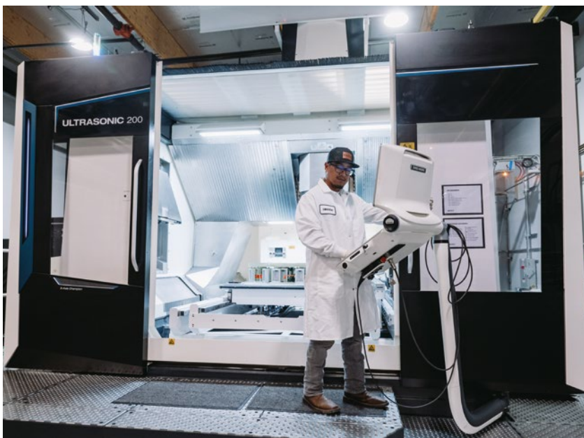
The ULTRASONIC 200 Gantry offers travels of 4,000×2,000×1,200 mm. The stable foundation of the gantry construction is an optimal basis for the high-precision processing of the mirror segments
