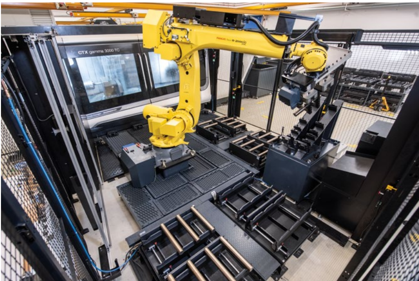
The CTX gamma 3000 TC, automated with MATRIS, produces high-precision spindles.
