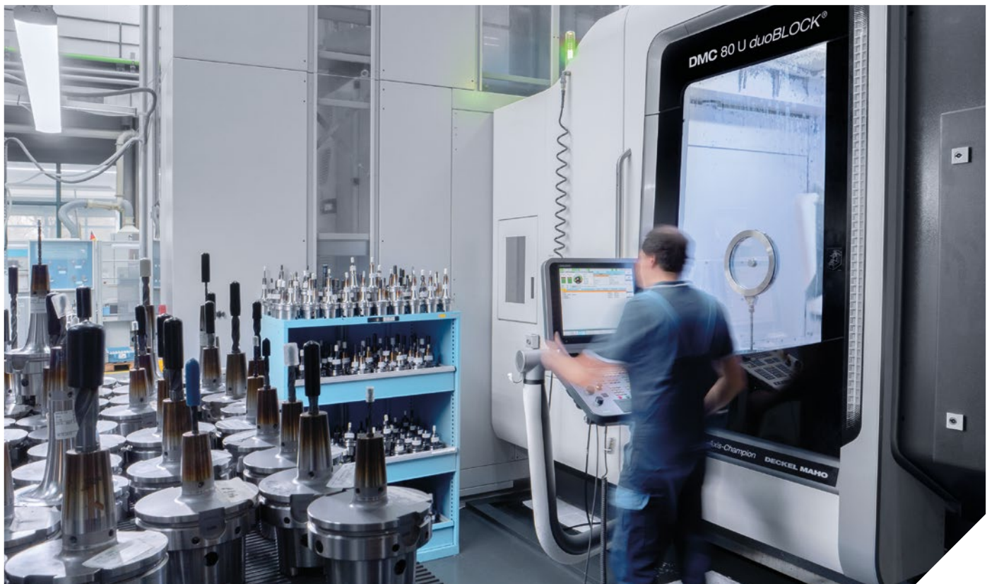
Components made of titanium, steel and aluminum are machined on two pallet pool systems, among others.
