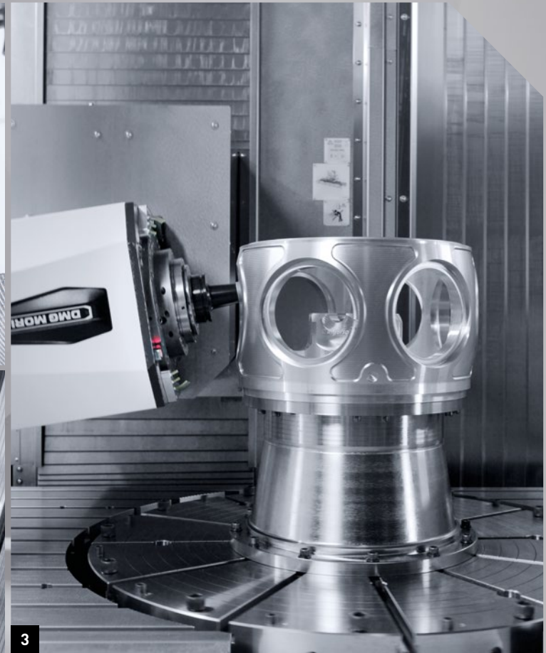
1. Machining CK45 with cutter head 100 mm (F: 1,500 mm/min; APP: 9 mm) 2. Machining of a gear wheel with DMG MORI technology cycle gearMilling 3. Mill-turn machining at up to 700 rpm and a maximum workpiece weight of 1,200 kg
