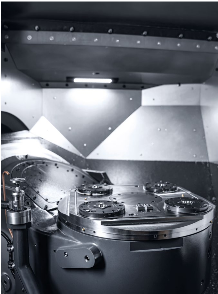
For optimal use of the working space, the two DMU 60 eVo machines have an MTS zero point clamping system embedded directly in the table.
