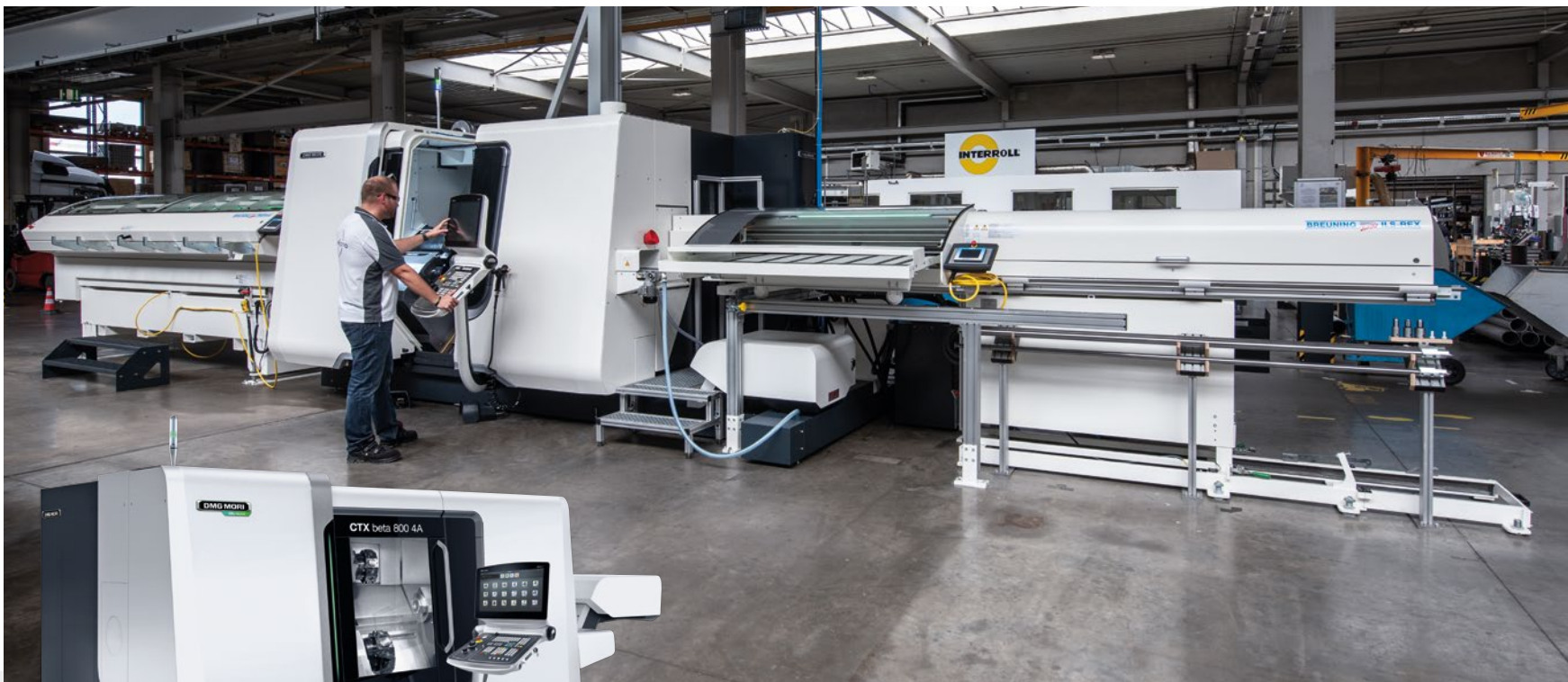
On the CTX beta 800 4A, Interroll manufactures components for drum motors fully automatically from loading to unloading.
