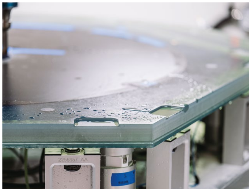
Assembly functions, such as sensor pockets, are also incorporated into the workpiece.
