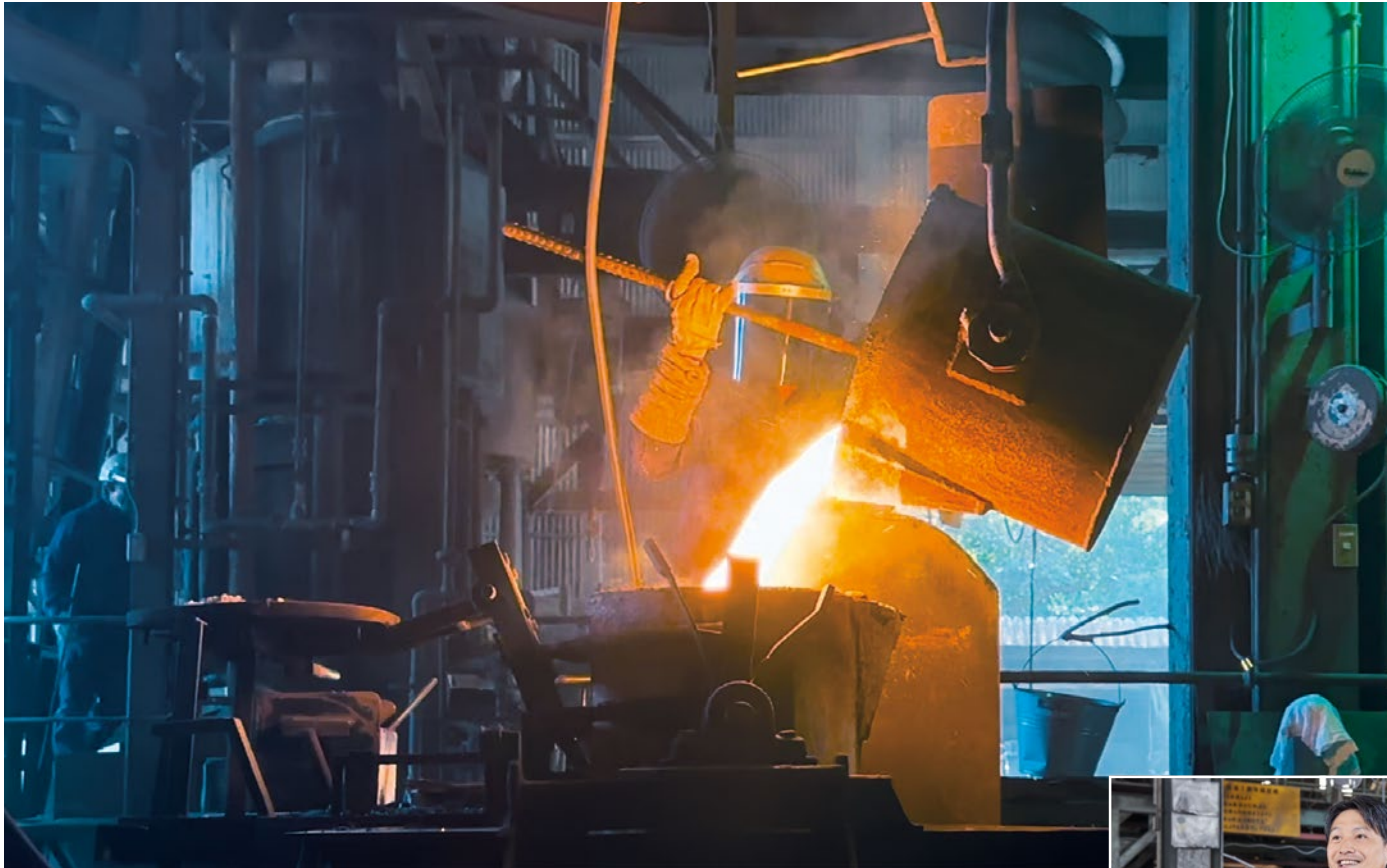
Casting process by metal melting and pouring at temperatures exceeding 1,000°C.
