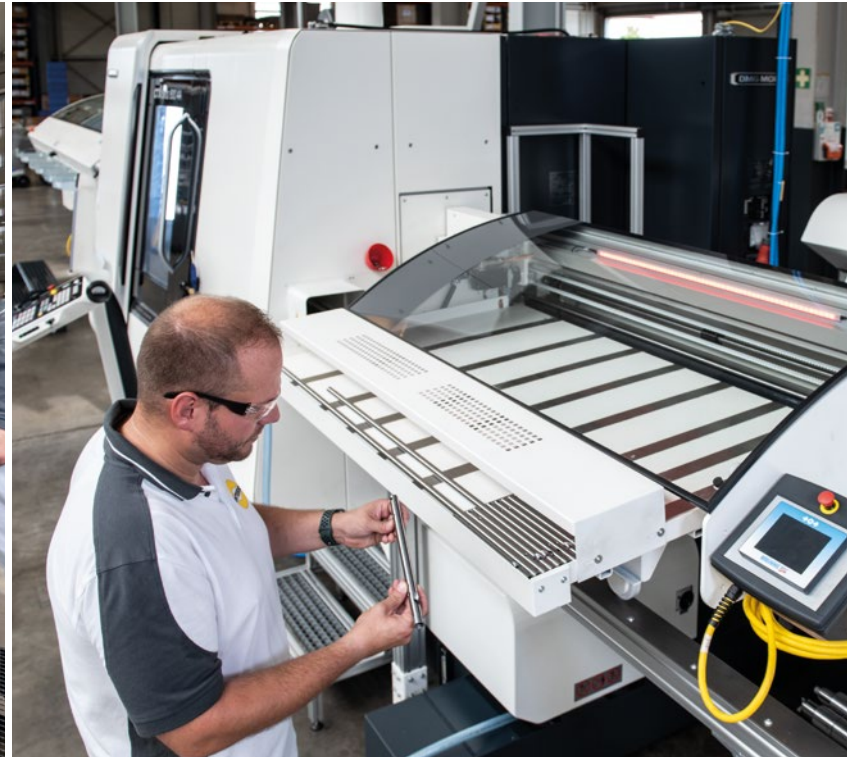
Longer workpieces are output through the right hand spindle of the CTX beta 800 4A and collected in the unloading system.
