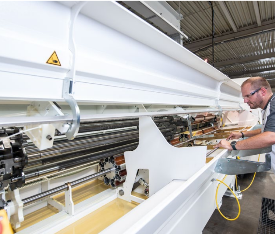
The bar feeder has eight guide channels so that the machine can process different jobs flexibly.
