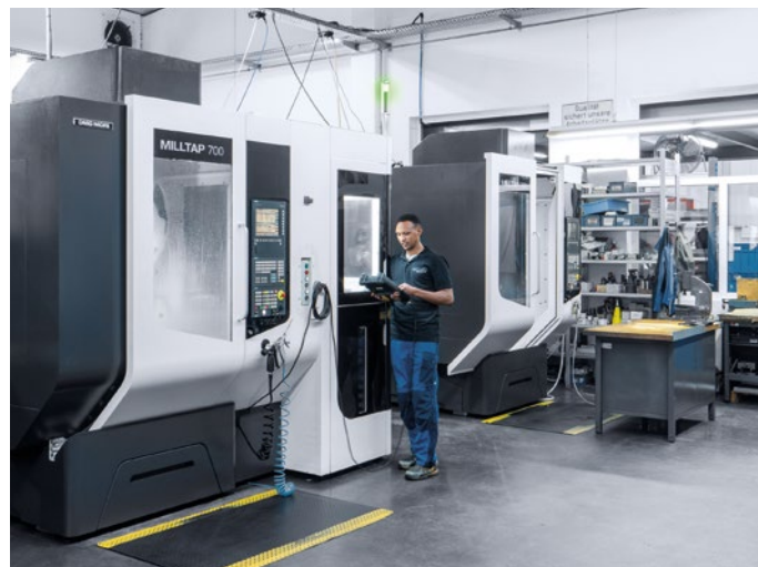
The MILLTAP 700 is used at Mechanik-Moduls for 5-axis machining of smaller workpieces. It is automated with a WH 3 Cell.
