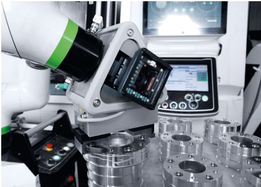
Vision Camera automatically detects the workpiece location and adjusts the arm motion to continue production regardless of misalignments.
