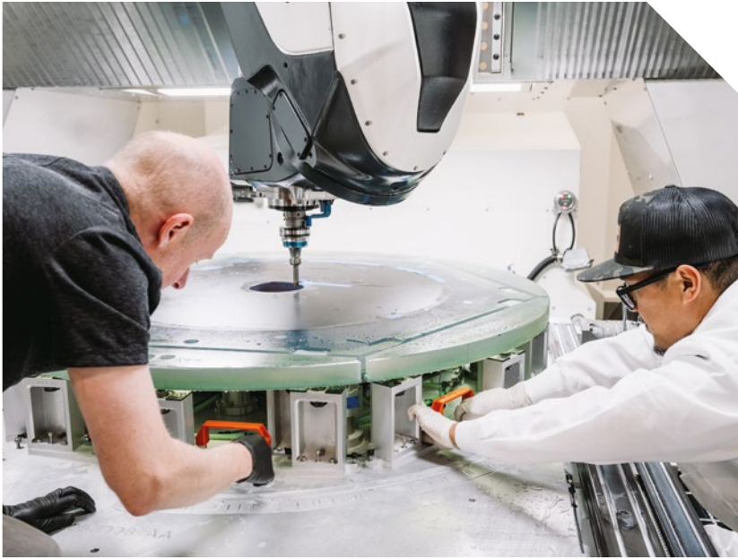
The engineers at Coherent developed a proprietary fixturing approach that uses a combination of support and clamping systems to fix the component.
