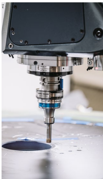
In ULTRASONIC machining, the diamond tool oscillates along its axis at a high frequency and low amplitude – in addition to the tool's own high-speed rotation.
