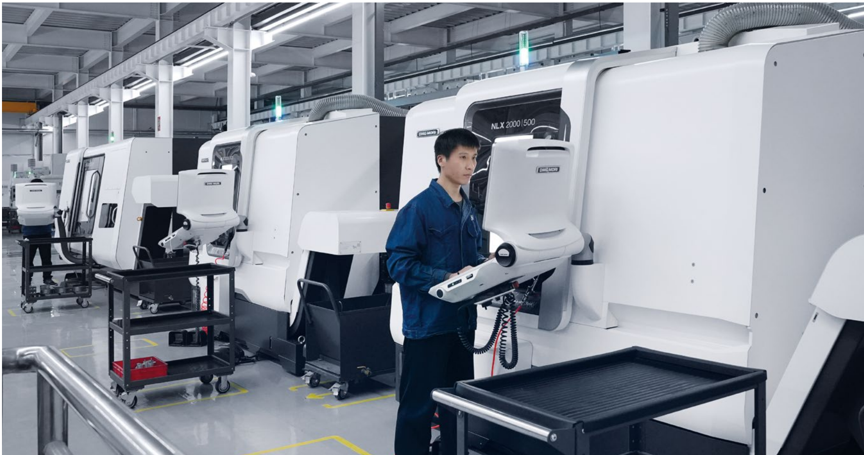
GRANDE-TEK Flow Control Co., Ltd. specializes in the development and manufacture of flow control systems and valves. Two NLX 2000|500 centers and a CTX beta 1250 TC are among the machines used for turning and turn-milling.
